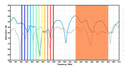
Operating principle of Wireless Multi-Channel Audio Systems. Instead of individual 200 kHz bandwidths as in narrowband transmission (left-hand side), the technology uses time slots in a 6 or 8 MHz wide window (right-hand side). More information at sennheiser.com/wmas
